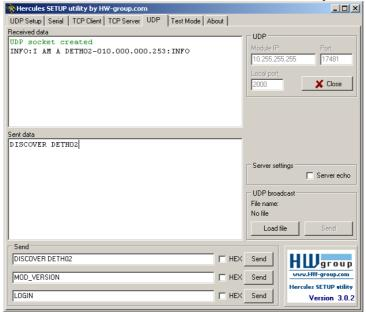
Now you know the exact IP address of the module (in this case 10.0.0.253). Close the connection and replace "Module IP" address with this one and click on "Listen". Send again the Discovery command to ensure that the parameters are correct. You can now send other commands to DETH02. You will find a summary of available commands with their answer.
