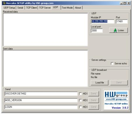
In this example, the DETH02 module is on a CLASS A Network (IP address like 10.x.x.x). If you are on a CLASS C Network (IP address like 192.168.x.x), the properties look like :
